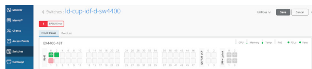
Figure 8: Wired Assurance BPDU Guard error
