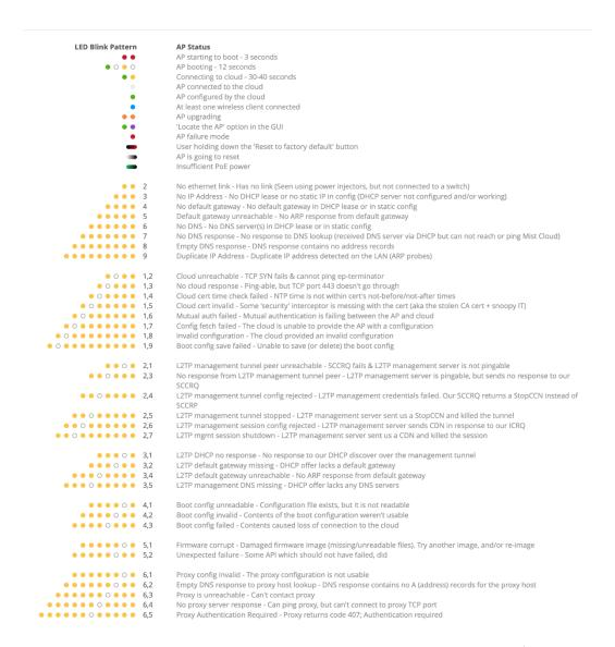
The first thing to do is to understand the source of the error by viewing the AP's status LED. If you can't see the LED on the AP, reboot it. If the AP is powered by PoE, then you can reboot it by using one of the two following methods:
