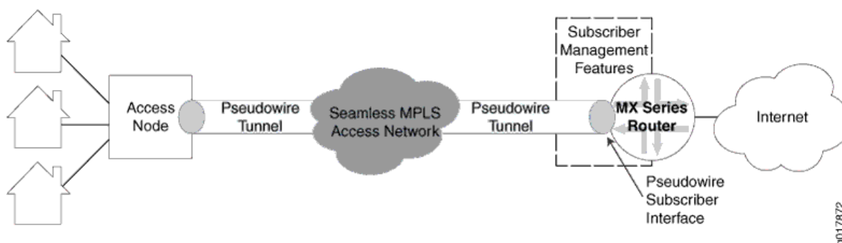
Figure 20: MPLS Access Network with Subscriber Management Support
