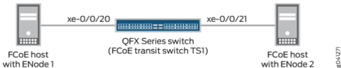
Figure 6: VN2VN_Port FIP Snooping (FCoE Hosts Connected to Same Transit Switch) Topology
