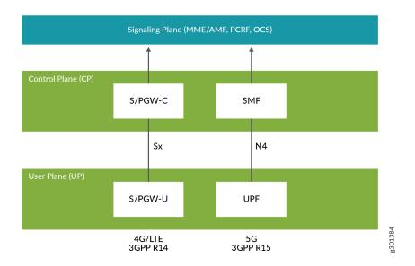
Junos Multi-Access User Plane supports MX routers functioning as user plane functions (UPFs) in accordance with 3GPP Release 15 CUPS architecture. The UPF provides high-throughput 5G fixed wireless and mobile wireless service in non-standalone (NSA) mode.
