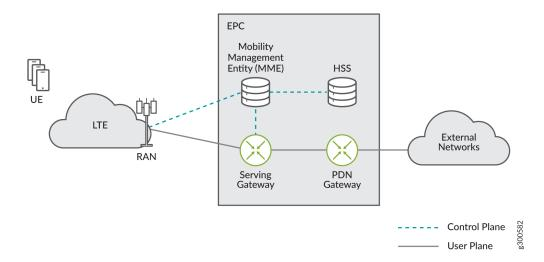
User Equipment (UE) has control path connectivity and data path connectivity to the EPC network elements over eNodeB base stations. The EPC provides data connectivity to external networks such as the Internet.
