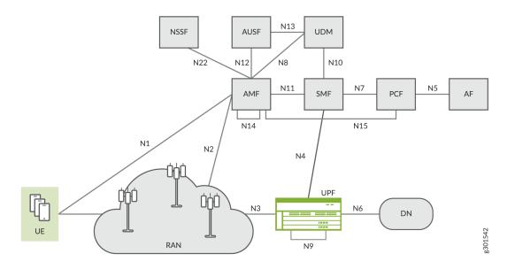
The 5G system architecture consists of the following network functions:
