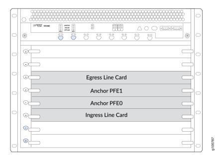
• The ingress line card provides the S1-U interface (SAEGW-U, SGW-U), the S5/8-U interface (PGW-U), or the N3 interface (UPF). The ingress line card also provides the Sxab interface (SAEGW-U), the Sxa interface (SGW-U), the Sxb interface (PGW-U), or the N4 interface (UPF).
