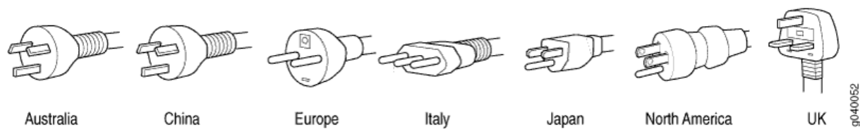
Figure 3: AC Plug Types
