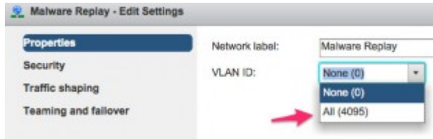
Figure 2: vSwitch VLAN Troubleshooting Config in port-groups
