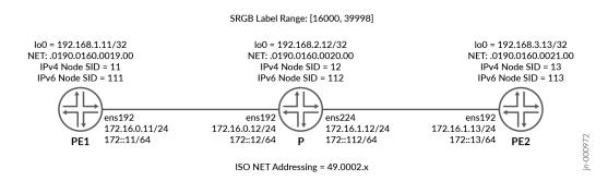
We want to segment routing in this network. PE1 is an ingress Cloud-Native Router node, P is a transit Cloud-Native Router node while PE2 is an egress Cloud-Native Router node. We will configure a common segment routing global block (SRGB) range for all nodes. All nodes are assigned a segment ID (node SID) for both IPv4 and IPv6.
