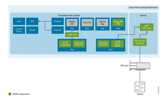
Figure 2: Components of Juniper Cloud-Native Router (eBPF XDP Datapath)
