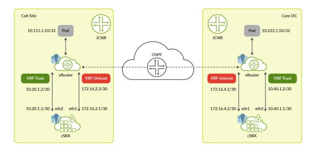
The topology consists of a Cloud-Native Router on the cell-site and a Cloud-Native Router in the core data center. Both JCNRs are service chained with cSRX. The core data center can also have any other physical or virtual firewall function as the tunnel endpoint. The traffic between pods 10.111.1.10 and 10.222.1.10 must be encrypted through an IPsec tunnel. The IP addresses and gateway addresses for the cSRX-Cloud-Native Router interface are also illustrated.
