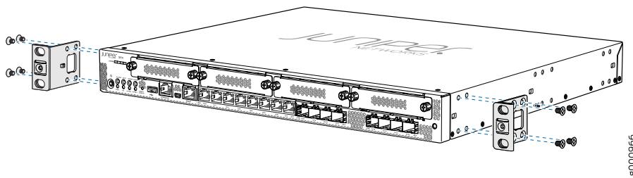
4. Lift the SRX340 and position it in the rack. Line up the bottom hole in each mounting bracket with a hole in each rack rail, making sure that the SRX340 is level.
