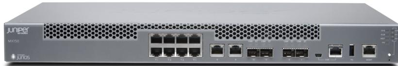
The MX150 has eight 1GbE RJ-45 network ports, two 1GbE RJ-45 access or uplink ports, two 1GbE SFP ports, and two 10GbE SFP+ ports. You can manage the router through an 1GbE RJ-45 management port, mini-USB console port, and an RJ-45 console (**CON**) port. The MX150 is shipped with a built-in AC power supply, and fans with front-to-back airflow.
