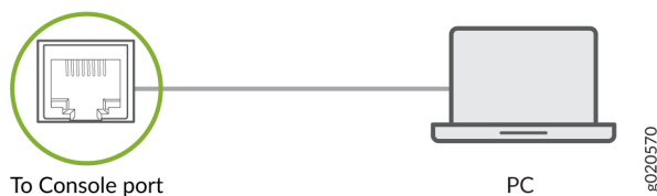
Figure 27: Connecting a Switch Directly to a Management Console
