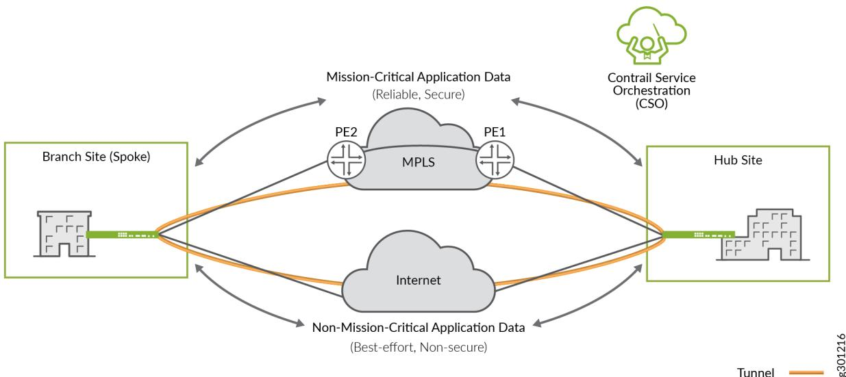
This example shows how SD-WAN is applied using CSO in a topology that has one branch site and one hub site. CSO builds one tunnel for the WAN links going over the MPLS network and a second tunnel for the WAN links going over the Internet.
