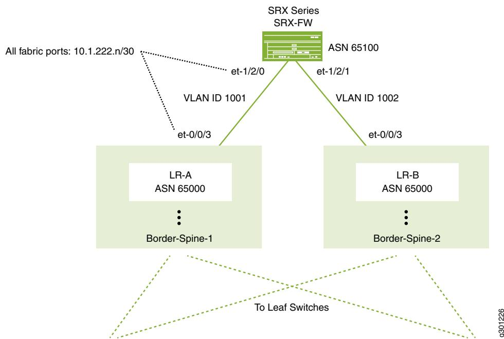
Before you begin, physically connect the SRX Series firewall to both spine switches (in a centrally routed and bridged model). Make sure the SRX Series device is already up and running and contains basic configuration such as a username and password, hostname, management and loopback IP addresses, but no IP addresses on the interfaces that you'll use to connect to the fabric nor any policies that govern traffic to and from the fabric.
