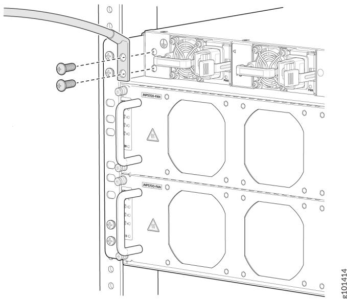
12. Connect the other end of the grounding cable to a proper earth ground, such as the rack.
