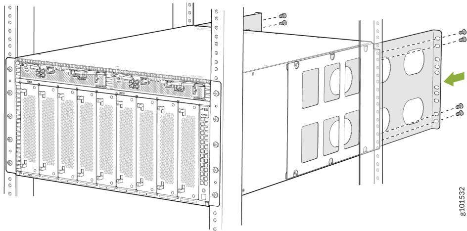
9. Secure the mounting blades to the rack rails using the rack mount screws (and cage nuts and washers, if your rack requires them).
