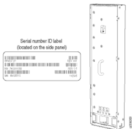
Figure 182: Standard-Capacity AC Power Supply Serial Number Label
