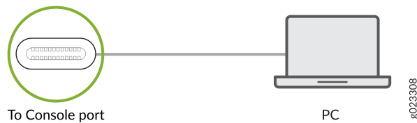
Figure 5: Connect Your Device Directly to a Management Console
