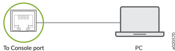
Figure 43: Connect Your Device Directly to a Management Console
