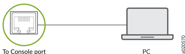
Figure 102: Connect a Device Directly to a Management Console
