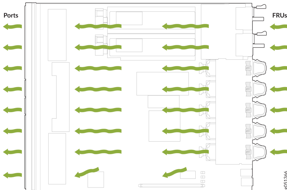
Figure 66: Back-to-Front Airflow Through the QFX5120-48YM Switch Chassis
