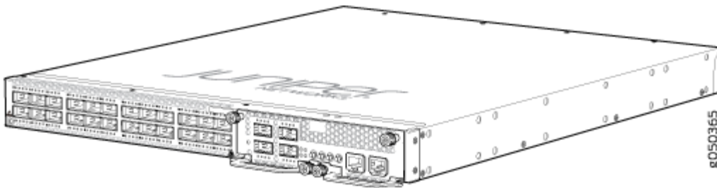
Figure 8: QFX5100-24Q-AA Port Panel with QFX-PFA-4Q
