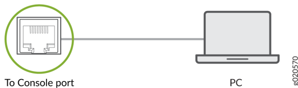
Figure 58: Connect a Device Directly to a Management Console
