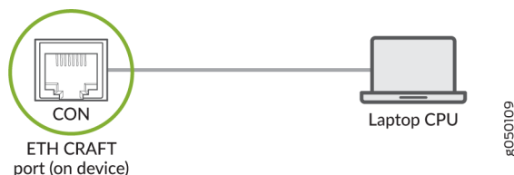
Figure 61: Connecting the PTX10003-80C Directly to a Management Console
