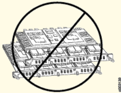
Figure 252: Do Not Stack FPCs
