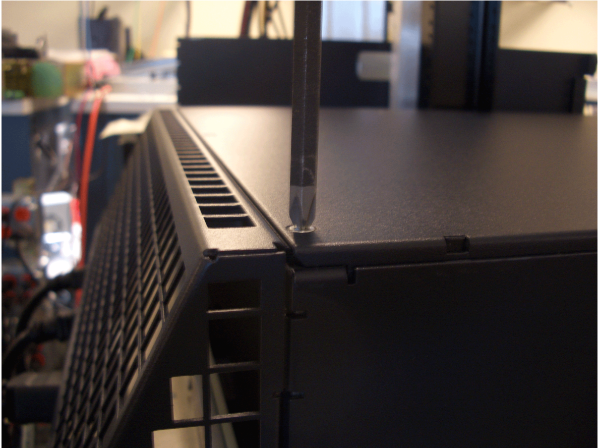
Figure 86: Removing the Top Right Screw of the Rear Air Exhaust Grate
