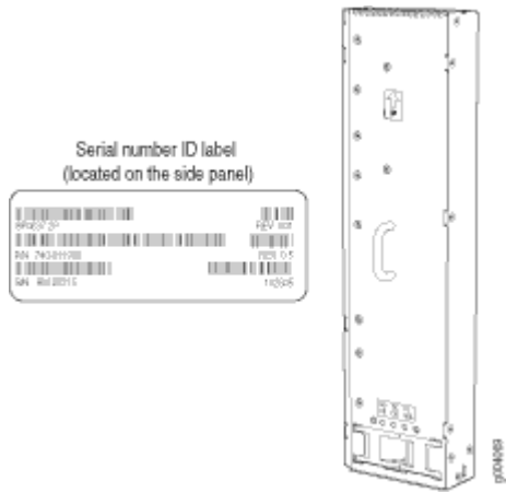
Figure 280: AC Power Supply Serial Number Label
