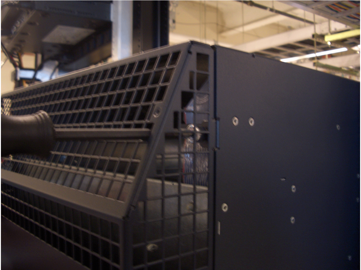
Figure 103: Tightening the Top Right Captive Screw of the New Rear Air Exhaust Grate
