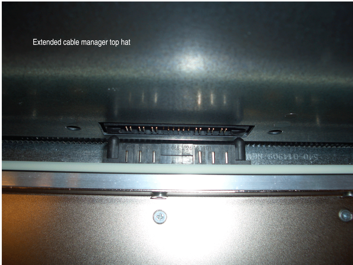
Figure 98: Fan Tray Connector on Extended Cable Manager Top Hat
