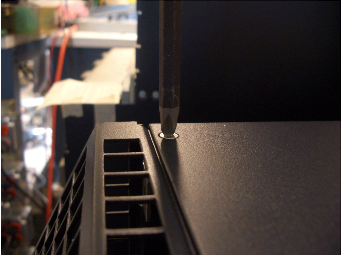
Figure 88: Removing the Top Left Screw of the Rear Air Exhaust Grate
