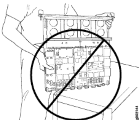
Figure 120: Do Not Rest the FPC on an Edge
