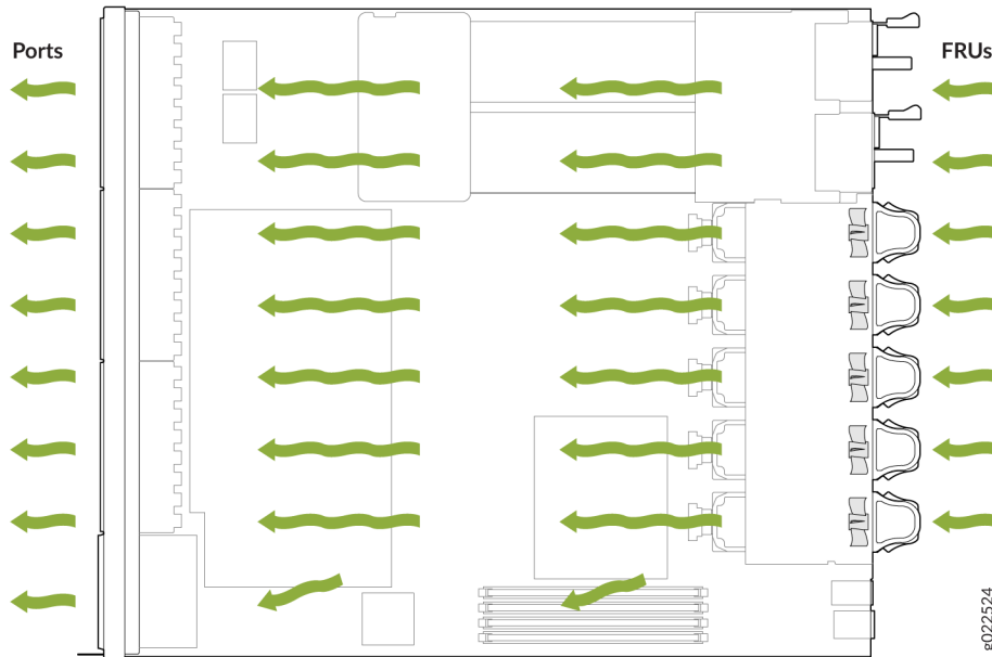
Figure 19: Back-to-Front Airflow Through EX4650 Switch Chassis
