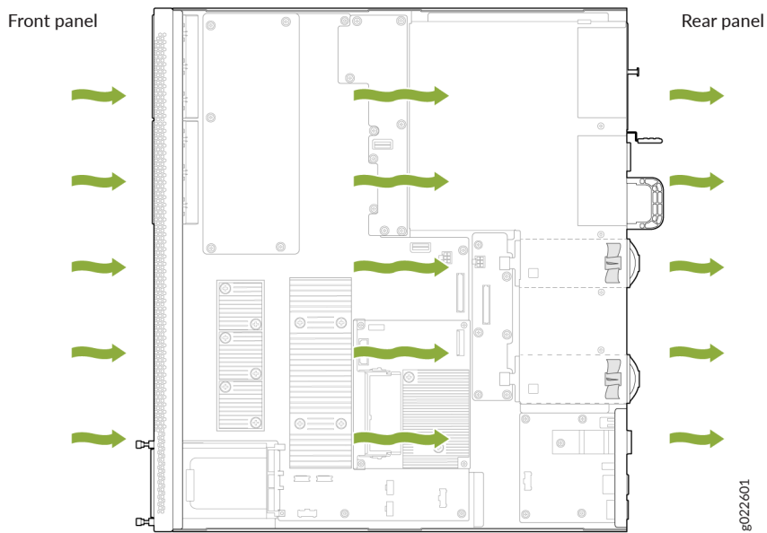
Figure 65: Front-to-Back Airflow Through an EX4400-24MP Switch Chassis
