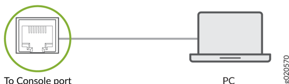
Figure 117: Connect a Device Directly to a Management Console
