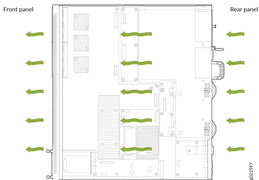
Figure 73: Back-to-Front Airflow Through an EX4400-24T Switch Chassis
