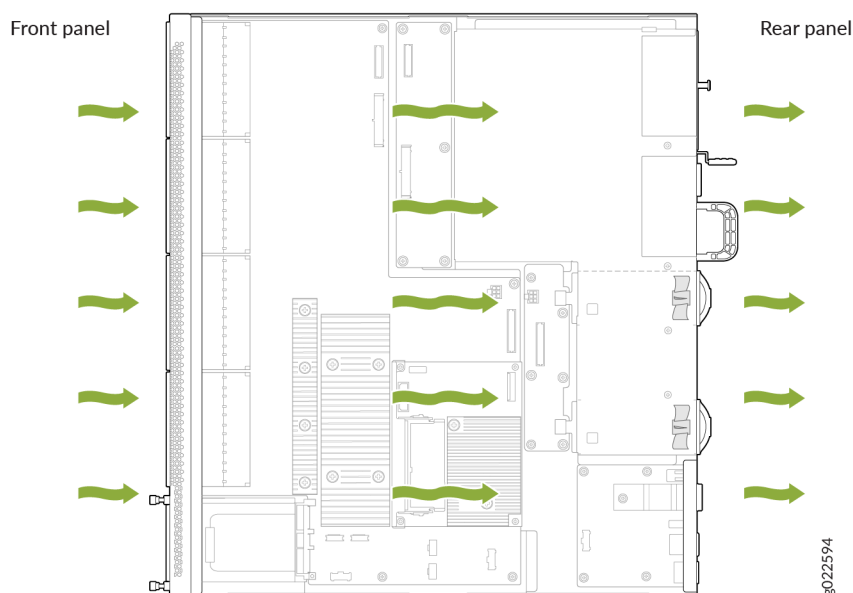
Figure 72: Front-to-Back Airflow Through an EX4400-48F Switch Chassis
