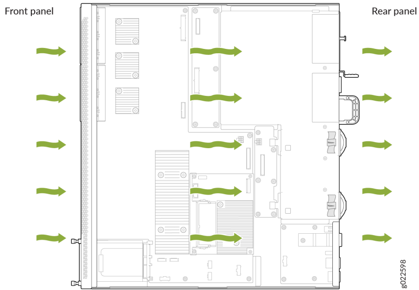
Figure 63: Front-to-Back Airflow Through an EX4400-24T Switch Chassis
