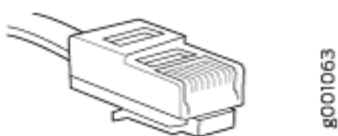
Figure 70: RJ-45 Connector on an Ethernet Cable
