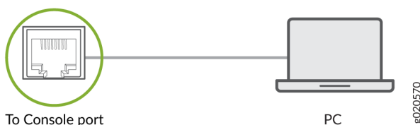
Figure 36: Connecting the ACX7509 Router Directly to a Management Console
