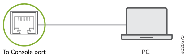
Figure 33: Connect the ACX7024 or ACX7024X Router Directly to a Management Console
