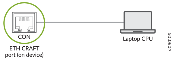
Figure 29: Connecting the ACX6360 Directly to a Management Console
