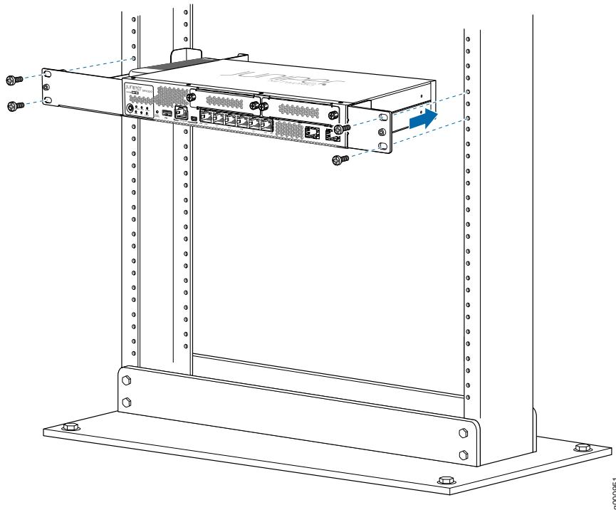
7. Check that the mounting brackets on each side of the rack are level.
