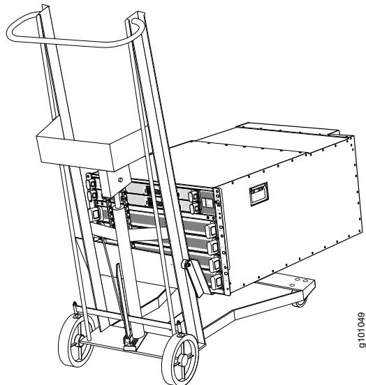
3. Align the router in front of the rack, centering it in front of the mounting tray.
