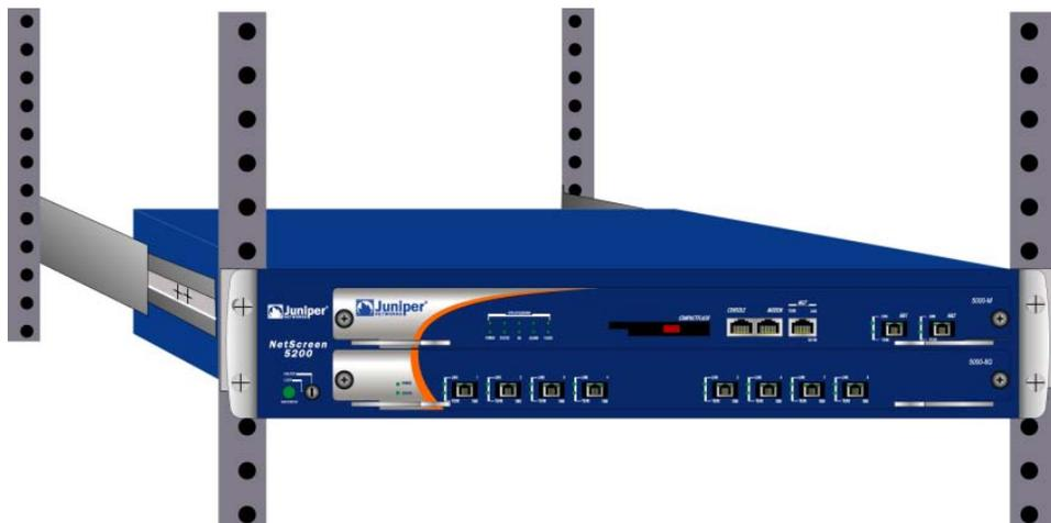
4. Screw the left and right brackets to the rack.
