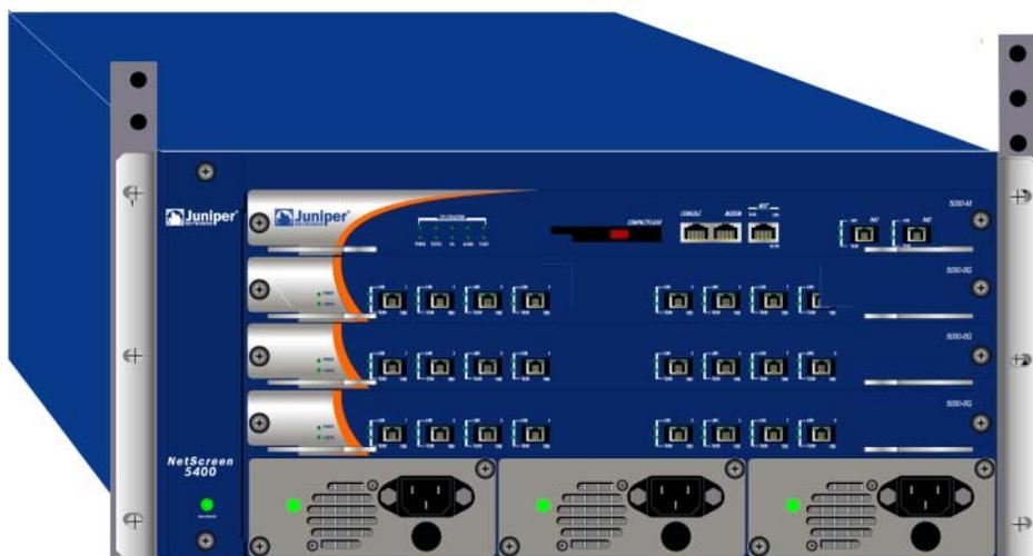
2. Screw the left and right brackets to the rack.
