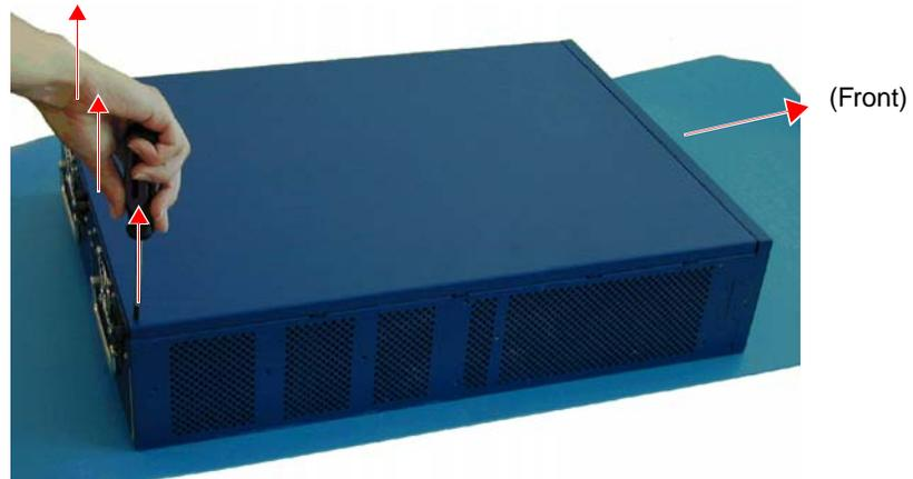
3. Grip the rear edge of the top panel, lift it up, and then remove it.
