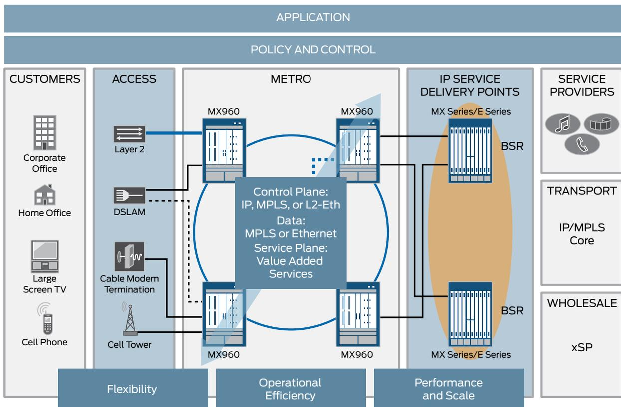
Figure 3: Universal Edge network architecture
