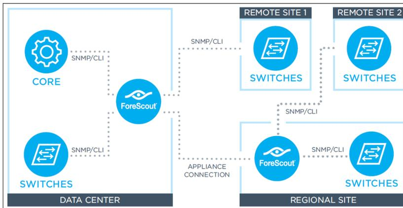
Figure 2: CounterACT communication with network devices
