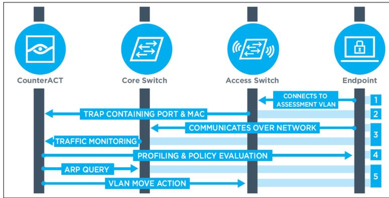
Figure 4: A sample CounterACT control flow
