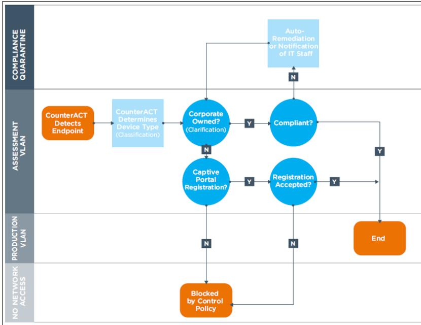
Figure 3: A sample wired pre-connect policy flow
