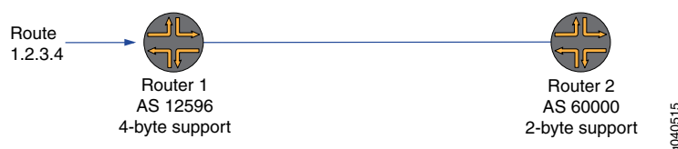
Figure 1: 4-Byte Capable Router Having a Peer Relationship With a 2-Byte Capable Router Using a 2-Byte AS Number
