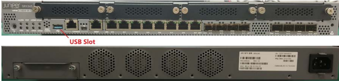
Figure 2-1: SRX340/345 Chassis different views
