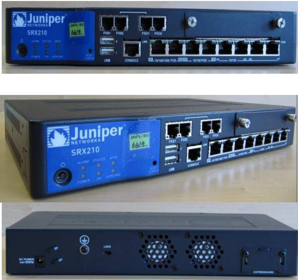
**Figure 2-1: SRX210H-P-MGW Chassis different views**
