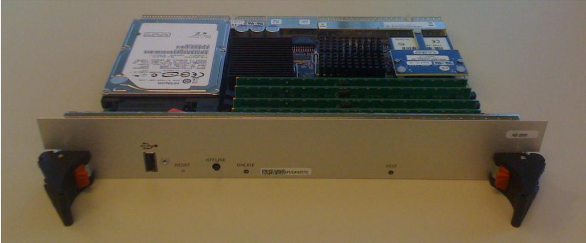
Figure 2-1: RE-A-2000 Routing Engine
