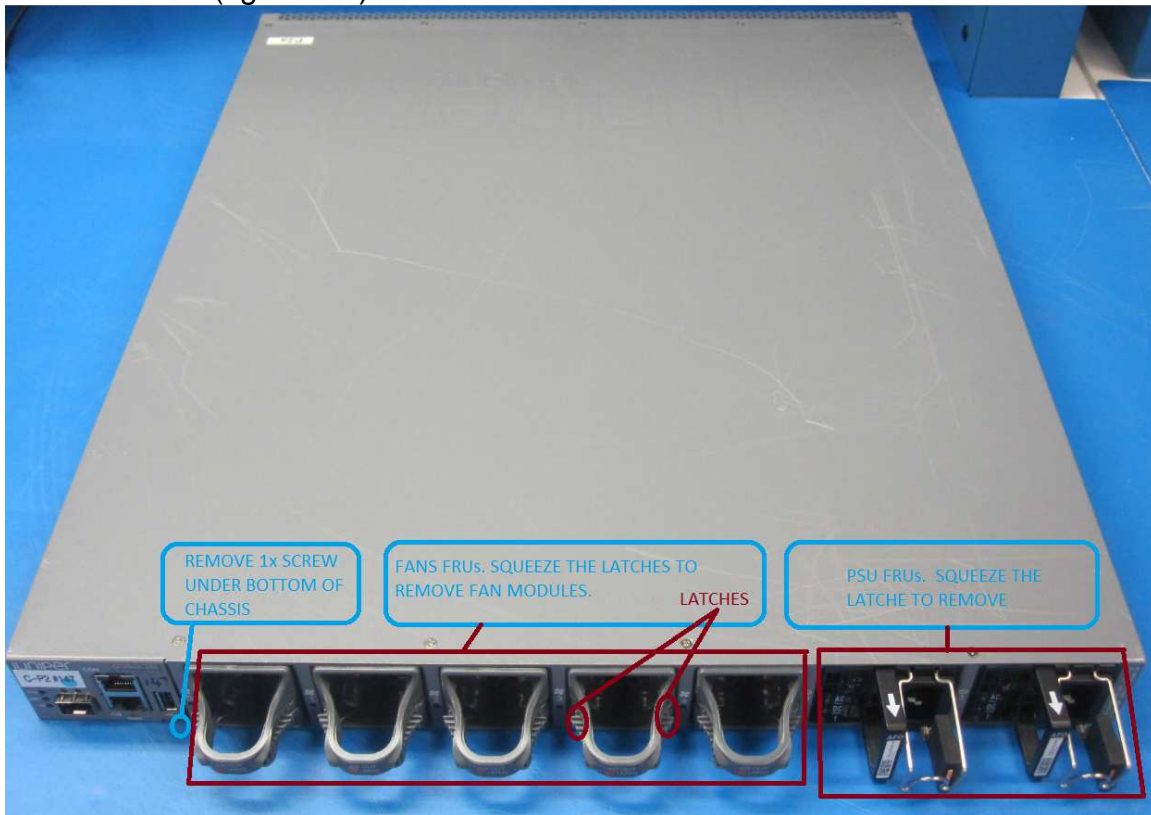
Figure 3-4: Rear screw + FAN FRUs + PSU FRUs
