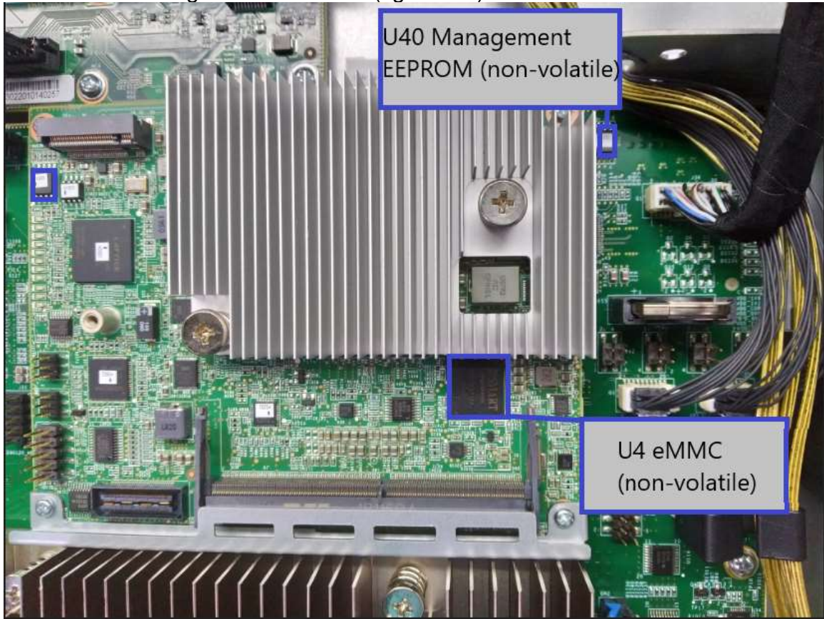
Figure 3-5: Locate NV storage (eMMC)
