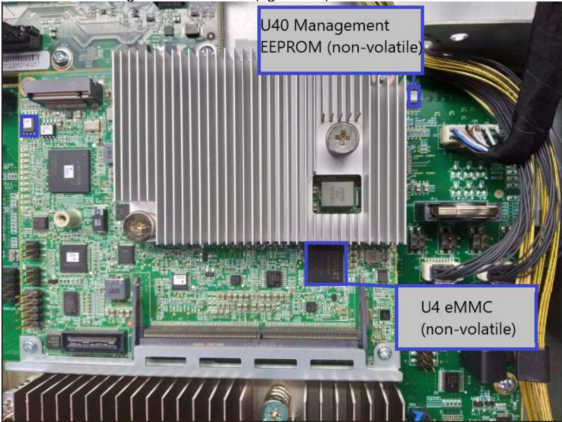
Figure 3-5: Locate NV storage (eMMC)
