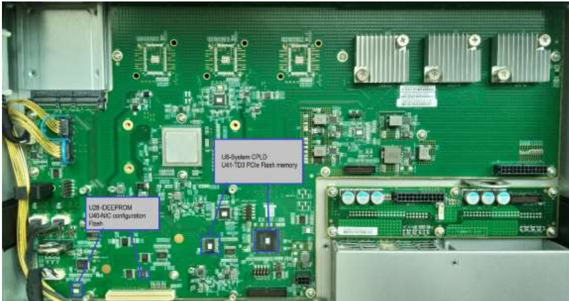
Figure 3-7: Locate System-CPLD, PCIe flash NIC IDEEPROM and MB-IDEEPROM.
