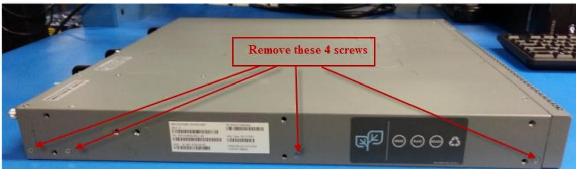
**Figure 3-2: Left side screws**
