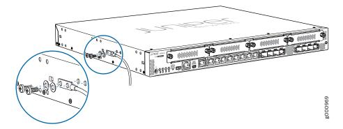
3. Secure the grounding cable lug to the grounding point with the screws.
