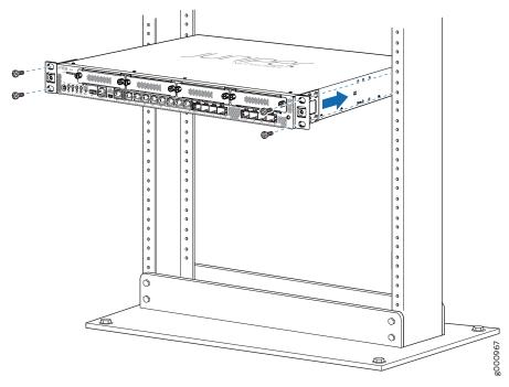
5. Verify that the mounting screws on one side of the rack are aligned with the mounting screws on the opposite side and that the device is level
