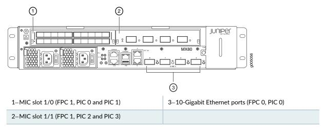
The chassis has two built-in MPCs, which are represented in the CLI as FPC 0 and FPC 1.
