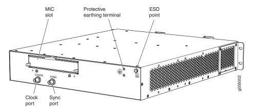
**NOTE**: The port labeled **CLOCK** provides 10 Mhz output. The port labeled **SYNC** provides 1 PPS output.
