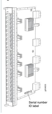
Figure 62: 2-Port MIC Serial Number Label
