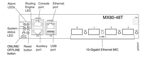
Figure 13: Front Panel on the Modular MX5, MX10, MX40, and MX80 Routers
