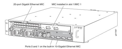
• MX80 router: Allows usage of all MIC slots (front and back) and all four ports of the built-in 10-Gigabit Ethernet MIC (labeled 0/MIC 0).
