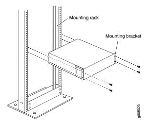
Figure 32: Installing the Center-Mounted Router in the Rack
