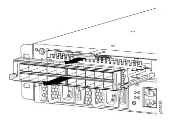
Figure 44: Removing a Dual-Wide MIC
