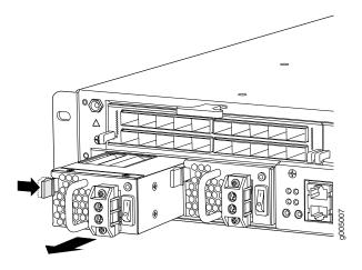
Figure 53: Disconnecting the DC Power Cables
