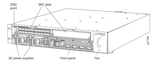
Figure 6: Front View of the MX10 Router
