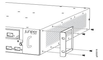
Figure 30: Center-Mounting the Brackets on MX5, MX10, MX40, and MX80 Routers
