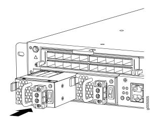
Figure 55: Connecting the DC Power Cables
