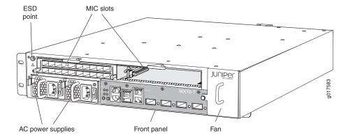
Figure 7: Front View of the MX40 Router
