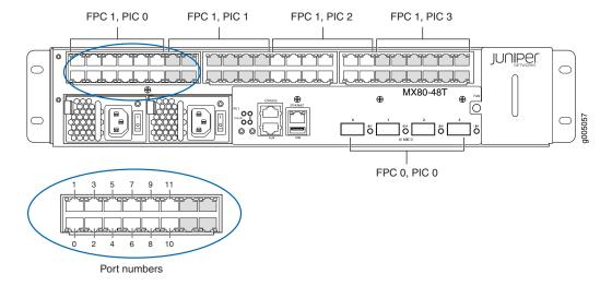
MPC 0 (FPC 0) contains a 4-port 10-Gigabit Ethernet MIC and is built into the front of the chassis. The MIC is represented as MIC 0 in the CLI and is logically divided into a single PIC, which is represented as PIC 0.
