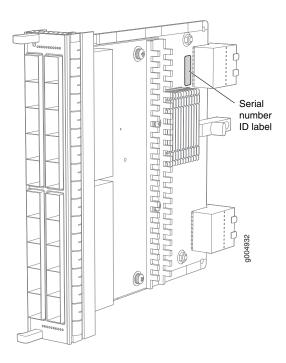
Figure 61: 40-Port MIC Serial Number Label
