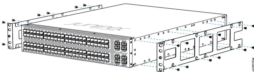
5. Attach the mounting rail to the switch using six mounting screws. Use cage nuts and washers if your rack requires them.
