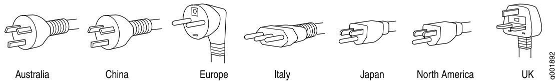
Figure 27: AC Plug Types
