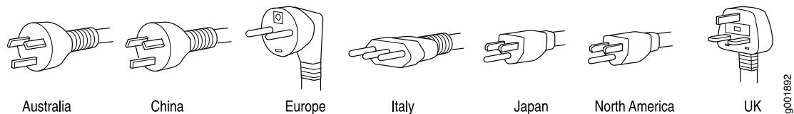
Figure 13: AC Plug Types
