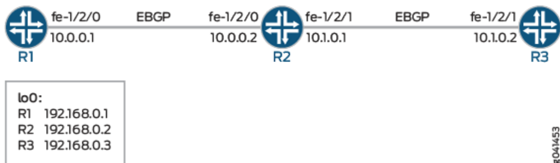
Figure 36: BGP Flap Damping Topology
